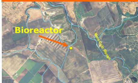
Water is pumped into the bioreactor from a collection point of three agricultural drainage ditches. This water then flows passively through the bioreactor to the outlet where it gravity feeds into the Seamist wetland. From there water flows into the Moro Cojo Slough, before joining the Old Salinas River. The Old Salinas River flows out to the Pacific Ocean at Moss Landing Harbor, where it also meets and mixes with water entering Elkhorn Slough during incoming tides.
